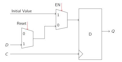
We now have a loadable D flip flop which is capable of remembering its state, loaded with new values, and initialized with certain values. The idea is that whenever Reset is 1, we grab the initial value regardless of the value of EN. But when Reset is 0, we behave like a D flip flop with enable.
