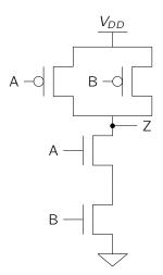
Here, there are two input bits, A and B, and one output bit, Z. We can check the following properties:
