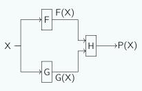
This circuit has three submodules F, G, H, and the latency of this circuit, also known as the propagation delay, is the sum of the times along the slowest path in the circuit. So if we have a latency of  $t_{PD}$ , then the combinational throughput will be  $\frac{1}{t_{PD}}$  (that's how many outputs per second we can produce).
