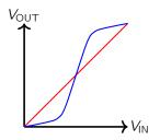
The two endpoints are **stable** here (representing the behavior when we feed in a 0 or a 1), while the middle point is **metastable** – that last point is something we'll return to later in the lecture.
