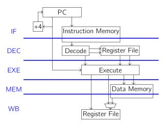
As a clarification, this means that we provide the data value associated with an address **during the next cycle** (if we have a cache hit), rather than in the same cycle. Clocked reads actually **simplify some pipelining issues**, which is why we're using them going forward.
