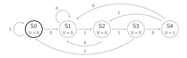
We give each state a name (S0 through S4), and each state has an associated output. (In this case, only being in S4 will allow us to unlock the lock.) We put a heavy circle around the initial state to indicate that it is where we
