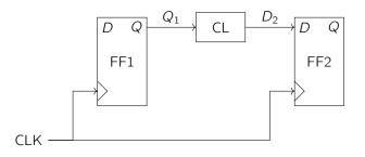
Then we need to make sure that the input  $D_2$  is stable at least  $t_{SETUP}$  before the next rising edge of the clock, but before that can happen, we need our bit D to propagate through our first flip flop FF1, which then goes through the combinational logic. So we need at least  $t_{PD, FF1}$  from the first flip flop, plus some time  $t_{PD, CL}$  to turn a stable Q1 into a stable D2, to all happen early enough. In other words, we need the inequality
