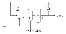
First, we use the reset RST component to initialize our state to 0. Then every time we want to increment our counter, setting inc to 1 allows the circuit to propagate forward that cycle using the wire with the "+1" instead of the wire without it. Here's what this implementation looks like in Minispec:
