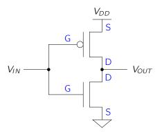
If we want to understand what this circuit computes, we start by labeling the diffusion terminals, which we've done in blue. This is easiest to do if we put the source voltage at the top of the diagram and the ground voltage at the bottom, as we've done here.
