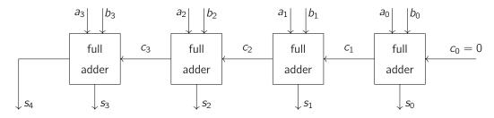
This is called a **ripple-carry adder** – it's simple and it's the cheapest adder in terms of area, but it's **slow** because of the series connections, and thus the propagation delay adds up across the n full adders. We'll see how to optimize this (to scale as log n instead of n) soon, but for now let's go back to the (one-bit) full adder and understand it more clearly.
