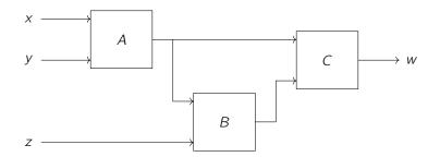
This device is indeed a combinational device as long as A, B, C are combinational devices, because we have digital inputs and outputs, and we can derive a functional description by writing out the function f in terms of the functions of the devices  $f_A$ ,  $f_B$ ,  $f_C$ : it will be
