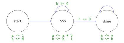
So at each cycle, we're in one of these three states, and we transition between states and do operations based on the values stored in our registers.
