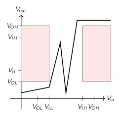
Even though the buffer is just supposed to copy over the input value, it's not good enough to just copy the voltage from  $V_{in}$  to  $V_{out}$  because of noise. And note that our VTC needs to avoid the **forbidden zones** which are shaded above: those are the regions where we feed in a valid input, but we end up with an invalid output.
