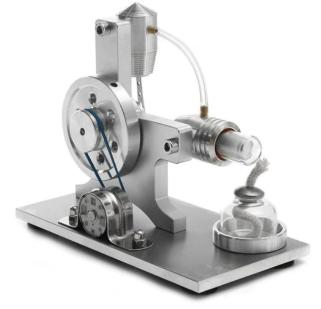
How does a heat engine work, generally? In principle, we can just say that we have a gas that compresses and contracts with a piston. But in this case, when we heat up the gas in the hot reservoir, a piston system actually moves the gas to the cold reservoir, where it cools down! We have pistons 90 degrees out of phase, and that lets our motor run.
