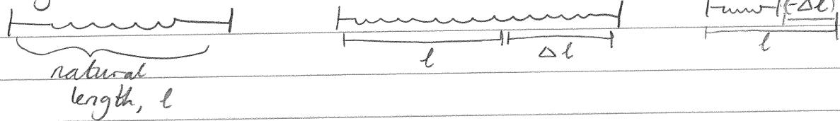
The extension of a spring is in direct proportion to the load applied to it.
