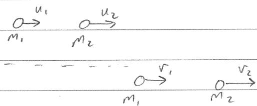
In an elastic collision the total kinetic energy is conserved.
