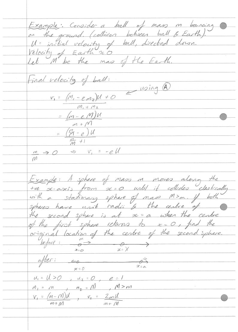
Let X be the initial position of the centre of M. At the collision, the centre of m is x-2(sum of 2 radii = 2) In the time T that M moves from X to a (with speed v2), m has moved from X-2 to O (with speed -v,) T = X-2 = a-X  $(X-2)v_2 + (a-X)v_1 = 0$ (x-2)(2my) + (a-x)(m-m)y = 0(=) X = (M-m)a + 4m d elastic e=1 M, = M2 = . - -  $u_1 = U_1, u_2 = 0, e = 1$  $v_1 = \frac{O+O=O}{2m} + \frac{1}{\sqrt{2}} = \frac{m(2)U+O}{2m}$
