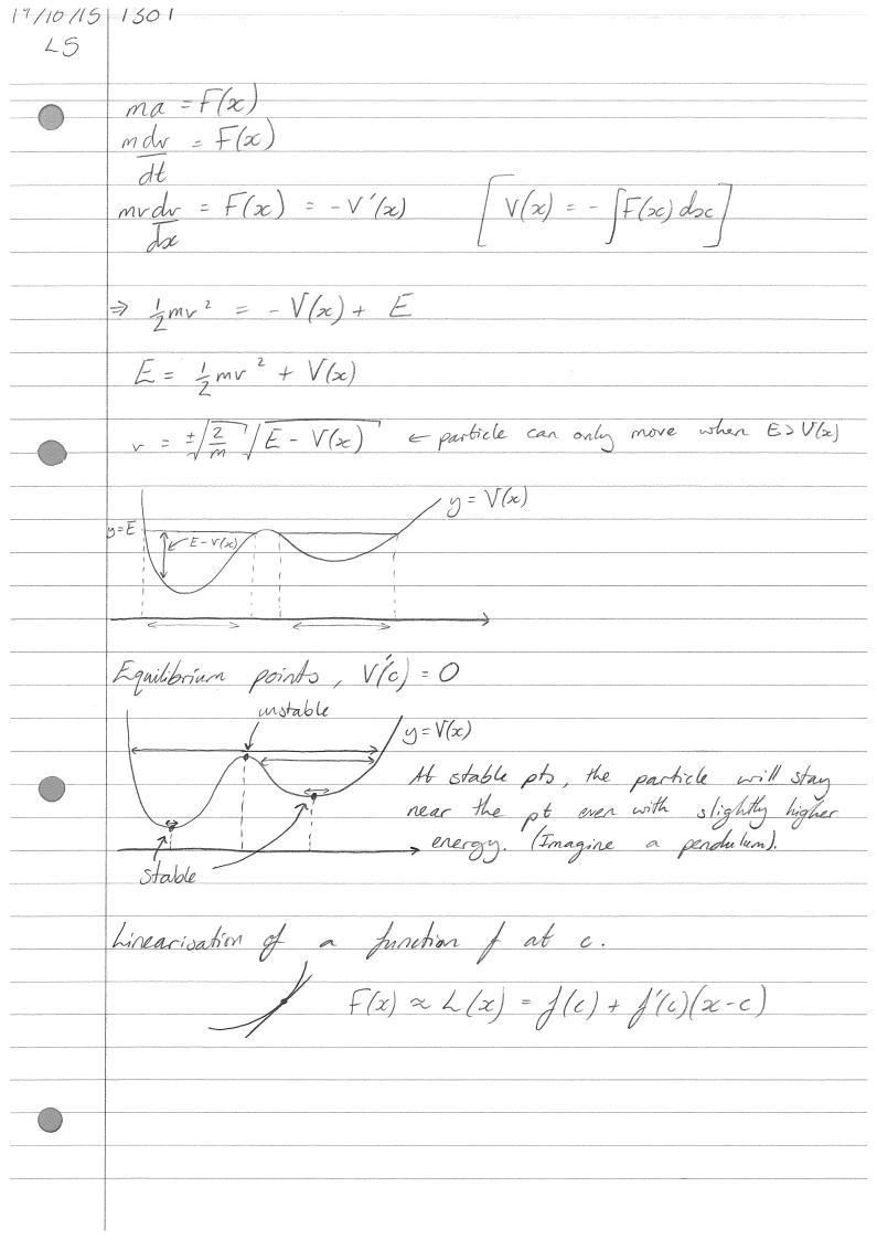
Let c be a stable equilibrium (a minimum) of V(x) s, t. V''(c) > 0 (NoT  $V(x) = xc^4$ ) Near x = c  $m\ddot{x} = F(x) = -V'(x)$   $\approx -\left(V'(c) + V''(c)(x-c)\right)$   $m\ddot{x} \approx -V''(c)(x-c)$ msic + V"(c)(x-c) =0  $\Rightarrow \ddot{X} + \frac{V''(c)}{m} \chi = 0$  $\dot{X} + \omega^2 X = 0$ ,  $\omega = \sqrt{V''(c)}$  $X = A sin(\omega t - d)$ period = 2 m So the period of small oscillations about x = c is approximately  $2\pi \sqrt{\frac{m}{V''(c)}}$
