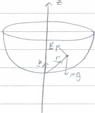
Because the surface is smooth, the reaction force is perpendicular to it.
