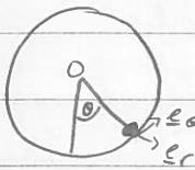
$$@ \text{cylinder smooth} \quad \underline{R} = -R \underline{e}_r$$
