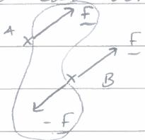
a force  $\underline{F}$  acting at  $B$ , plus a couple  $(a-b) \times \underline{F}$
