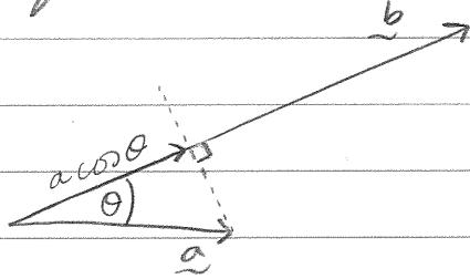
The part of  $\underline{b}$  cut off by the perpendicular is the projection of  $\underline{a}$  onto  $\underline{b}$ .
