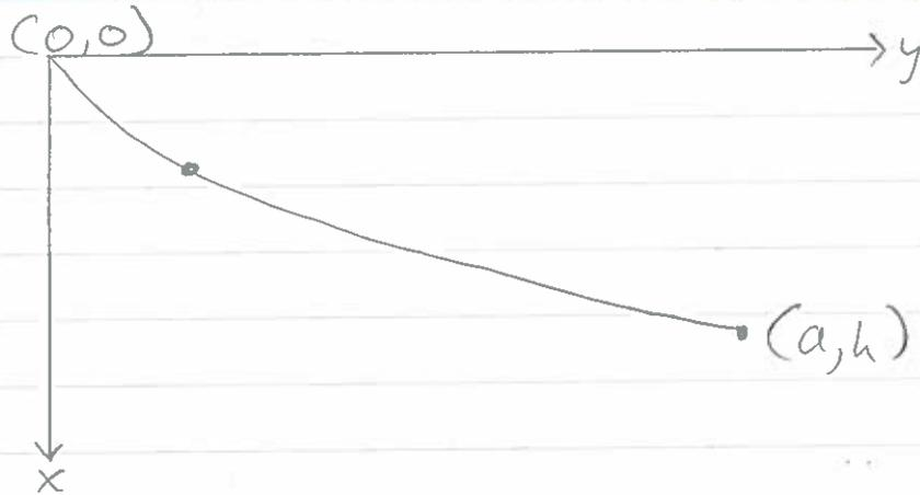
Find  $g(x)$  such that the time taken for a bead to fall due to gravity from  $(0,0)$  to  $(a,h)$  on wire  $y(x)$  is a minimum.
