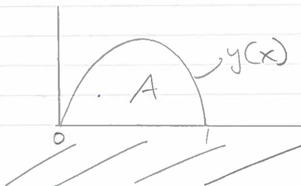
$$L = \int_0^1 \sqrt{1+(y')^2} \, dx \quad \begin{array}{l} y(0) = 0 \\ y(1) = 0 \end{array}$$
