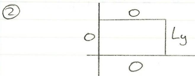
$$\nabla^2 \phi = 0, \quad \phi = X(x) Y(y).$$
