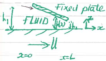
Angle  $\alpha$  (small), axes fixed in the plate; pressure  $p$  is atmospheric ( $p_0$ ) outside the gap
