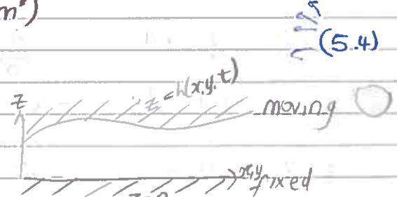
$$So u = \underbrace{\frac{p_x}{2\mu} z(z-h)}_{\text{PPF}} + \underbrace{\frac{h_z}{h}}_{\text{CF}} \quad \text{with } u=0, z=0 \quad \left. \begin{array}{l} u=u, z=h(x, y, t) \end{array} \right\} \text{b.c.} \quad (5.5)$$
