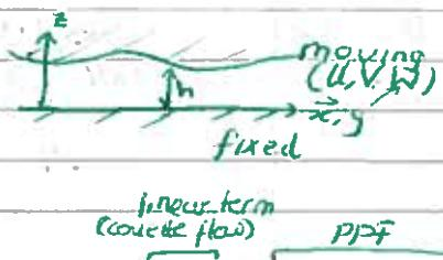
(lubrication approximation), we can integrate to get  $U = \frac{U_z}{h} + \frac{P_x}{2\mu} z(z-h)$
