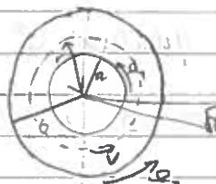
Couple exerted across any cylindrical surface of radius  $r$  is due to shear stress  $\sigma_{rz}$  acting on element of length  $r d\theta$ .
