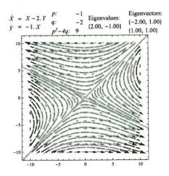
Only the two special straight line trajectories pass through (0,0). The others approach the critical point, from the direction of one of these straight lines and leave the critical point in the direction of the other. The critical point is known as a *saddle point*. A change in the sign of p interchanges the roles of  $\lambda_1$  and  $\lambda_2$  as before.
