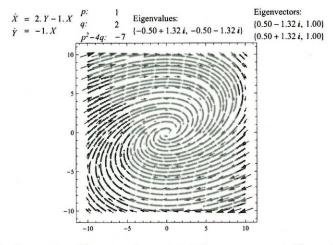
All trajectories approach the origin. The singular point is known as a stable spiral point or focus.
