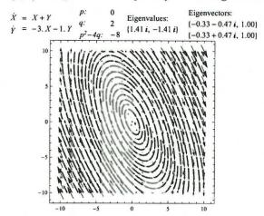
The critical point is called a *centre*. Again it is illustrative to pick out the lines Y = -3X and Y = -X and note that the individual trajectories have turning points on these lines.
