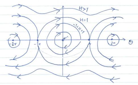
H = -1, trajectories consist of points  $\theta = 2n\pi$ , v = 0-1<H<1, trajectories are closed and 0 is restricted
