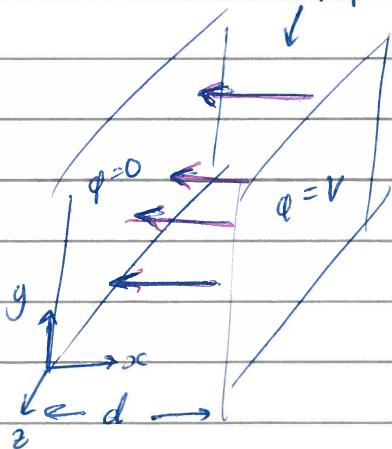
Plates held at  $\phi = 0, \phi = V$
