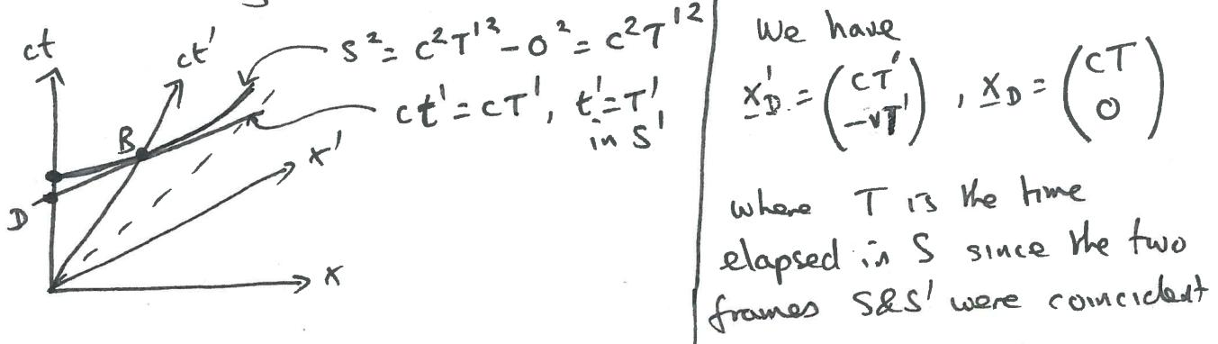
However  $T < T'$  since the point on the  $ct$  axis where it intersects with the hyperbola  $s^2 = c^2 T'^2$  corresponds to  $t = T'$  as  $s^2 = c^2 t^2 - x^2 = c^2 t^2 - 0^2 = c^2 T'^2$  at  $t = T'$ . As  $D$  is closer to 0 along the  $ct$  axis than is this point  $T < T'$
