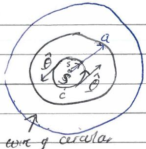
wire of circular cross-section with uniform current density  $J$ , directed out of the paper
