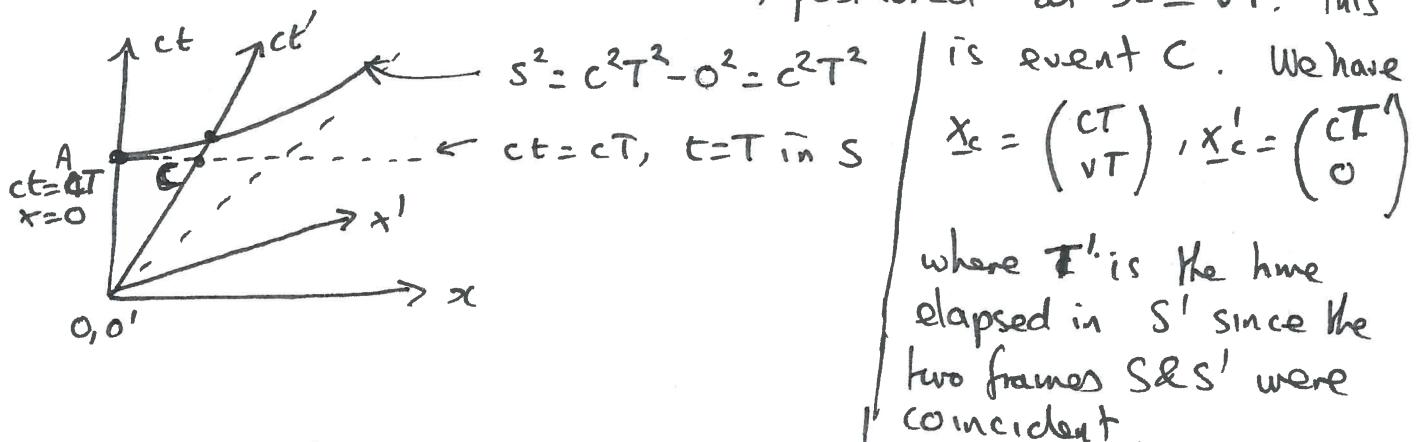
However  $T' < T$  since the point on the  $ct'$  axis where it intersects with the hyperbola  $s^2 = c^2T^2$  corresponds to  $t' = T$  as  $s^2 = c^2t'^2 - x'^2 = c^2t'^2 = c^2T^2 \Rightarrow t' = T$ . As C is closer to O' along the  $ct'$  axis  $T' < T$ .
