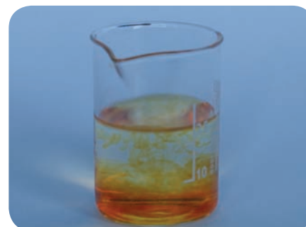
▲ This shows the red-brown colour you get when potassium iodide is oxidised by an oxidising agent.
