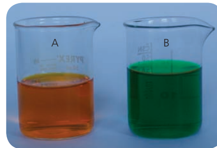
▲ A and B show the colour change from orange to green when potassium dichromate(VI) is reduced.
