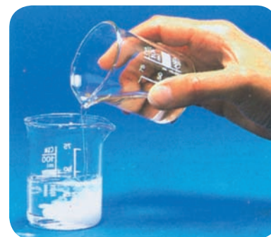
▲ The precipitation of barium sulfate.
