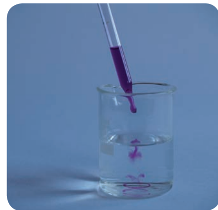
▲ Adding potassium manganate(VII) to an unknown liquid. The purple colour is fading, so the liquid must contain a reducing agent.
