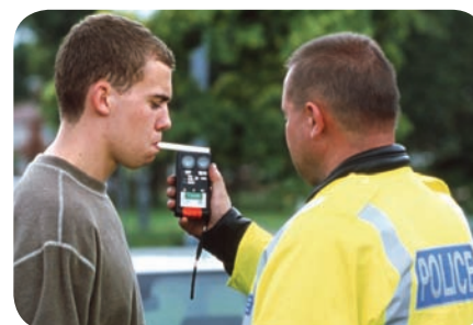
▲ A breathalyser test. The device contains potassium dichromate(VI), which is orange. Alcohol on the breath causes a colour change to green.
