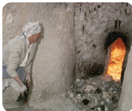
▲ Limestone (calcium carbonate) being heated in a lime kiln to give calcium oxide (called lime, or quicklime). The lime might be used to make limewash for buildings, or mixed with sand to make lime mortar.
