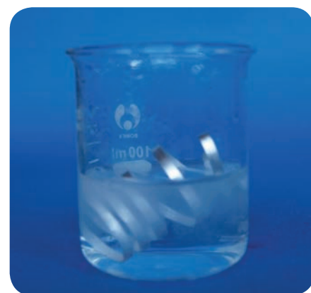
▲ Magnesium reacting with dilute sulfuric acid. Hydrogen bubbles off.
