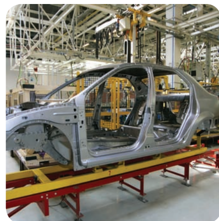
Zinc is coated onto steel car bodies, before they are painted, because zinc protects the steel from rusting, by sacrificial protection.
