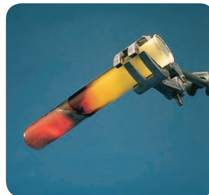
▲ Iron filings reacting with sulfur. You need heat to start the reaction off – but then it gives out heat.
