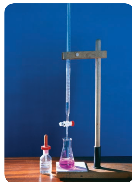
▲ A titration: sodium hydroxide solution was added to hydrochloric acid, from the burette. Neutralisation is complete: the phenolphthalein has turned pink.
